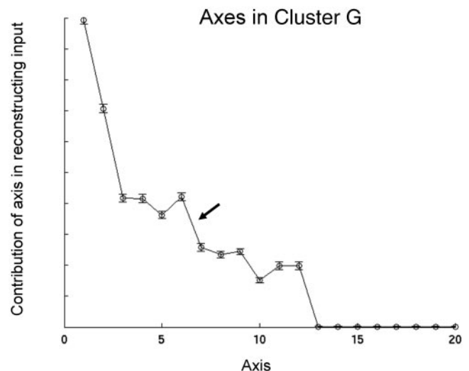
FIGURE 3. Contribution of axis versus axis number. The norm of A_m , on the y-axis represents the contribution of axis m in reconstructing the input. Note the small contribution of axes 7 through 12. There was no contribution after 12 axes.
