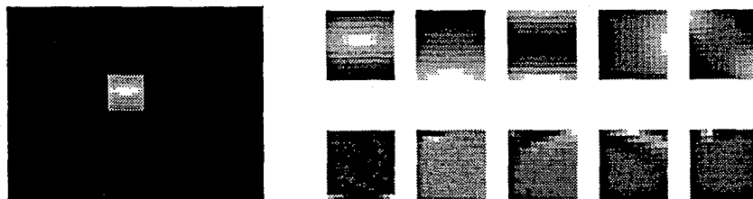
Figure 3: Left: Sample local image basis. Upper right: Local principal component filters ordered with first eigenpatch on left. Lower right: Local independent component filters ordered according to magnitude (shortest filter on left).
