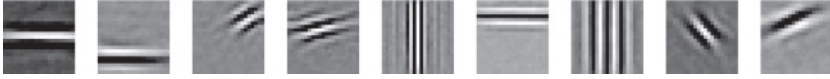
Figure 6: Examples of Gabor filters from ICA trained on position-centered patches. They are much more extended in space and wavelength than the conventional ICA results (see Figure 4).
