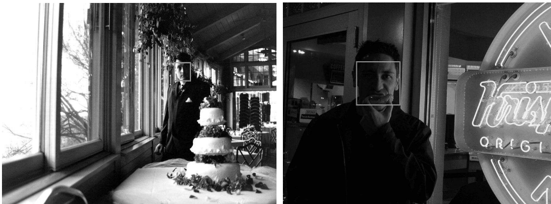
Figure 1. The face detector results for two complex background and illumination conditions. The system works in real time at 30 frames per second on a fast PC.
