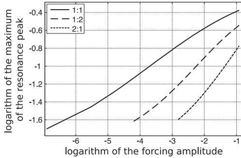
Figure 6: Power law for the maximum of the resonance peaks. Log of the resonance peak power for 1:1, 1:2, 2:1 as a function of the log of the forcing amplitude  $\epsilon$ . Network parameters as in Figure 4, right.
