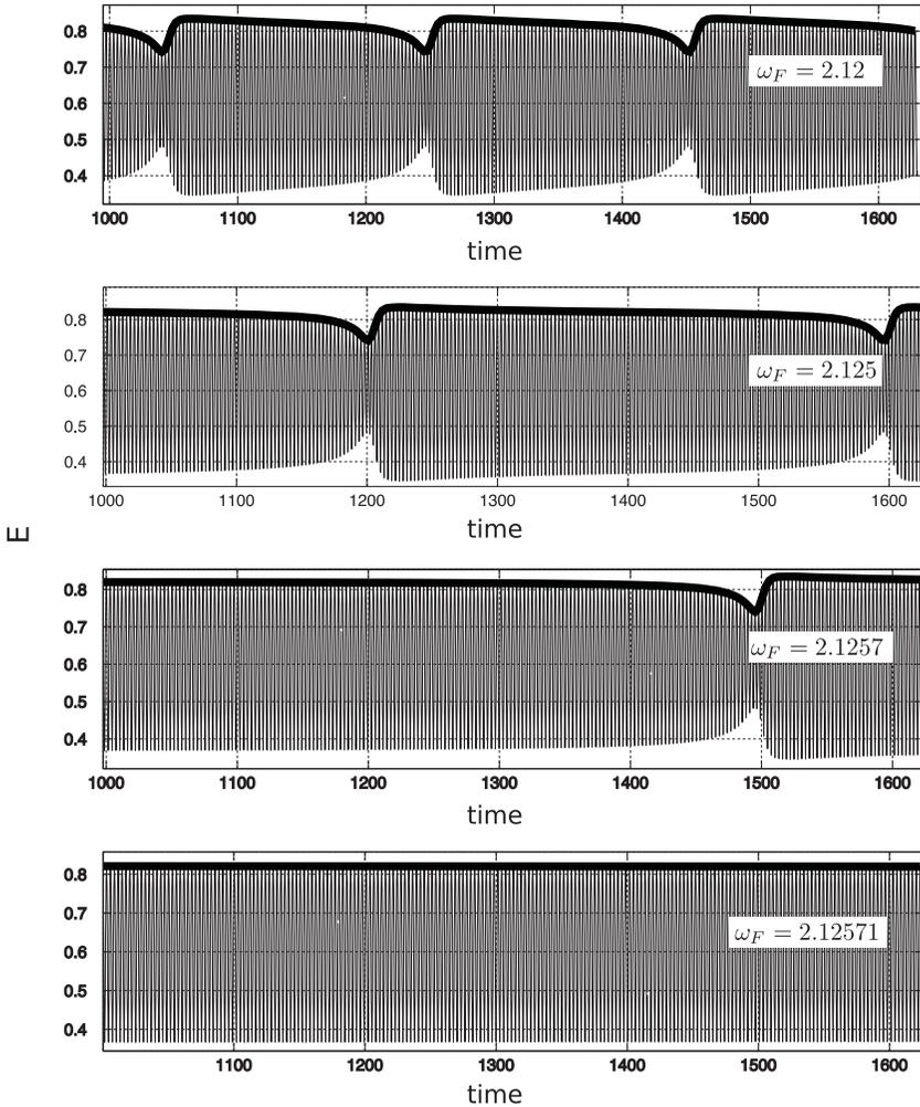
Figure 9: Example of convergence to a homoclinic response. Plot of the excitatory response for different forcing frequencies. The forcing parameters are such that the dynamics is close to the homoclinic curve. Different parameters from Figure 4, right, are  $\theta_i^{(0)} = 0.824174$ ,  $\epsilon = 0.05$ .
