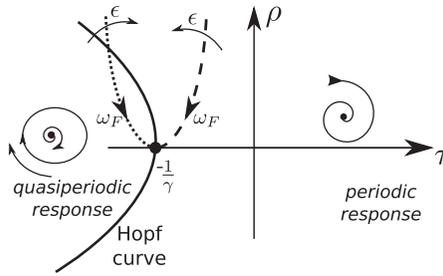
Figure 7: Dynamics for the amplitude of the network response in the case  $\epsilon_0 = -1$ . Bifurcation diagram of equation 3.6 in the plane  $(\tau, \rho)$ . The dashed curves are the resonance curves parameterized by the perturbation  $\delta\omega$  (dashed for the ISN regime, dotted for the SO regime). Adapted from Gambaudo (1985).
