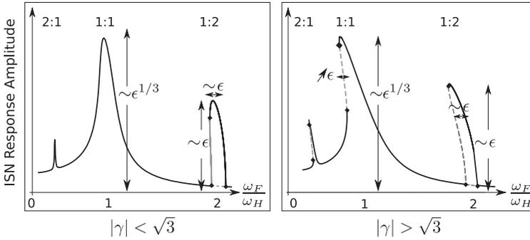
Figure 11: Plot of the resonance curves in the ISN regime for two different shears  $\gamma$ . The scaling of the width and amplitude of the peaks is indicated as a function of the forcing amplitude  $\epsilon$ . The domain of multistability for  $|\gamma| > \sqrt{3}$  is a decreasing function of  $\epsilon$  but an increasing function of  $\gamma$ . The amplitude of the 1:1 peak does not scale exactly as  $\epsilon^{1/3}$  as indicated. For more details, see the text and appendix F.
