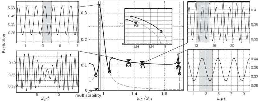
Figure 10: Example of resonance curve in the SO regime. Plot of the amplitude of the response as function of forcing frequency. The gray box shows one period of a periodic response. See the text for further explanation. Parameters:  $\epsilon = 0.01$ ,  $\delta\theta^{(0)} = -0.0018$ . Same network as in Figure 2. The torus solution is continued until the resonance R2 where the continuation fails. (Computed with Auto07p and Knut.)
